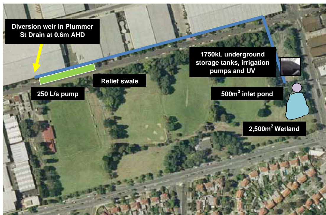
Figure 4-10 Schematic of preferred option for Murphy Reserve stormwater harvesting scheme
