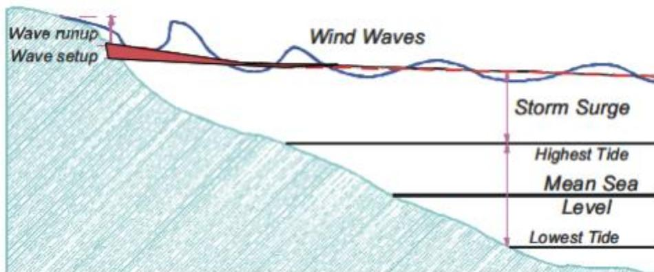
FIGURE F-10 WAVE SET-UP AND RUN-UP (CSIRO 2009)
