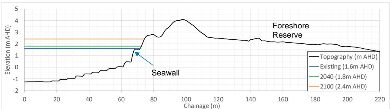
**FIGURE F-8 CROSS SECTION PROFILES 1 TO 4 (TOP TO BOTTOM) – PROFILE AND 1% AEP STORM TIDE LEVELS**
