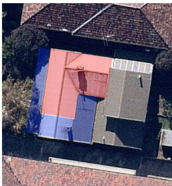
Figures 6 & 7 - Floor plan (left) and recent aerial photograph showing the front part of the house. The original extent of the three-roomed 1872 cottage is shaded red, and the 1890s additions are shaded blue. (Source: McGrath Real Estate and Nearmap)
