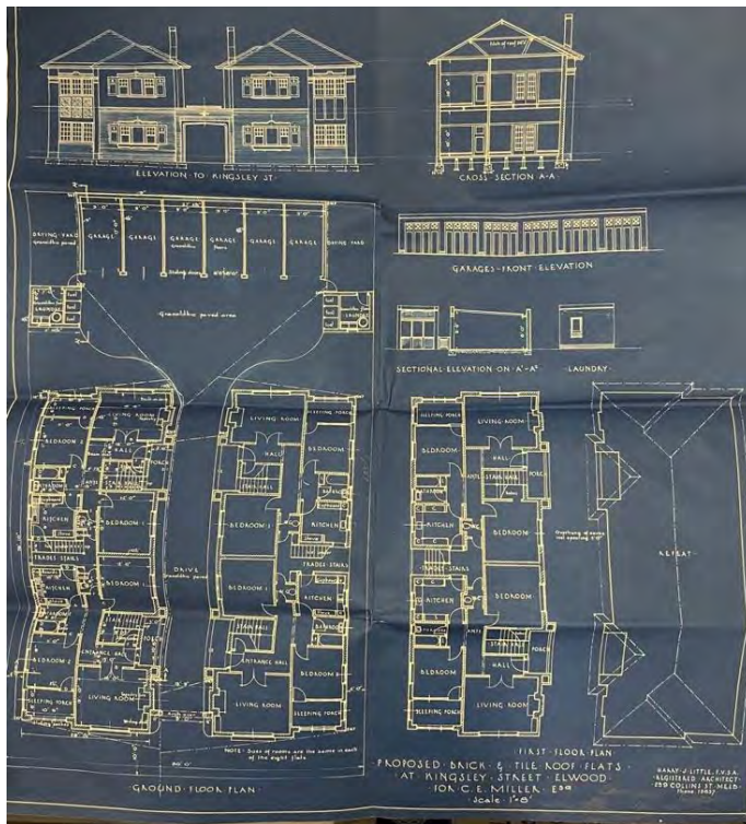
Figure 4. Proposed brick and tile roof flats at Kingsley Street, Elwood for C. E. Miller Esq (plans, elevation and section). Source: Harry J Little. n.d. Drawings of 4-6 Kingsley Street, Elwood. Council Records. City of Port Phillip.
