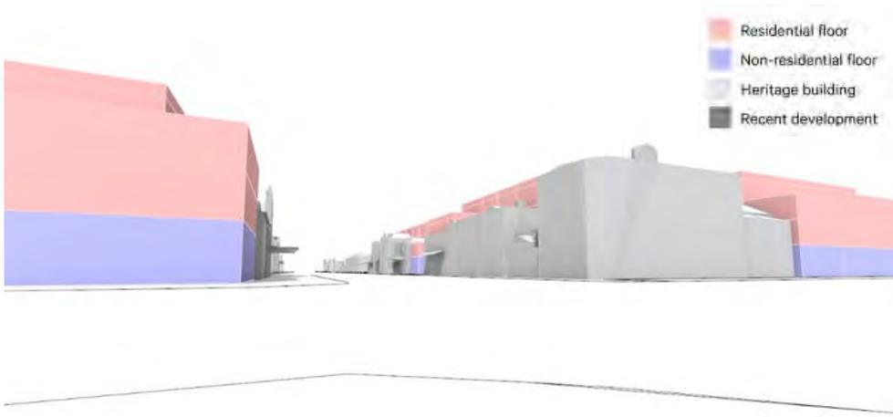
**Figure A25.** View 14: Northeast corner of Clarendon Street and Park Street, looking south along the western side of Clarendon Street. (HO440) 14.8m (4 storeys) mandatory maximum building height. 6m mandatory minimum upper-level setbacks to Clarendon and Park streets. Southeast corner site and infill along southern side of Park Street 11.6m (3 storeys) maximum street wall height is proposed.
